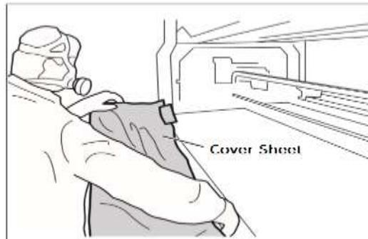
*Fig 29: Removing the Cover Sheet*
