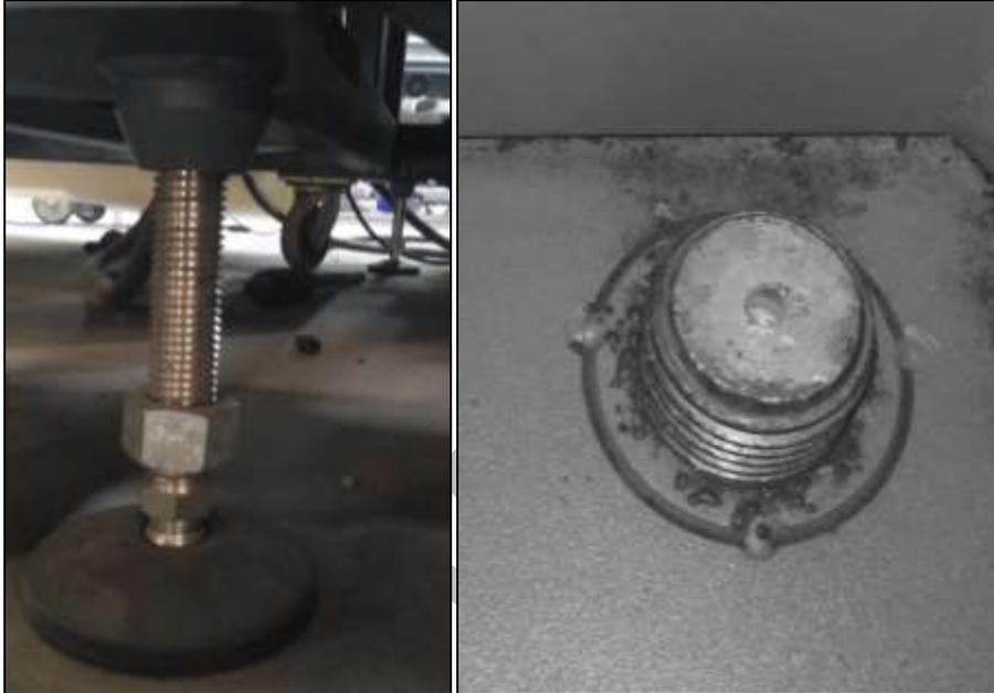
*Fig 3: Displaying the Main Machine Leveller*
